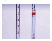
Pipette liquids with precision. Fisherbrand graduated class AS type 1 pipettes are made from soda lime glass. Type 1 pipettes have the zero mark at the top.
