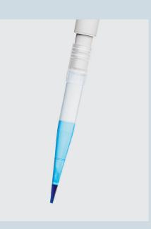
Residual liquid when pipetting detergent containing solutions
